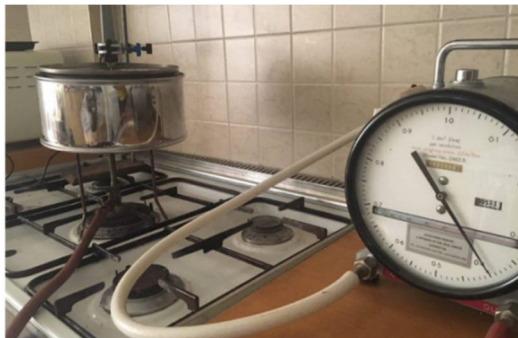
Figure 2. The experimental equipment including gasometer, Bunsen burner, and double wall container
