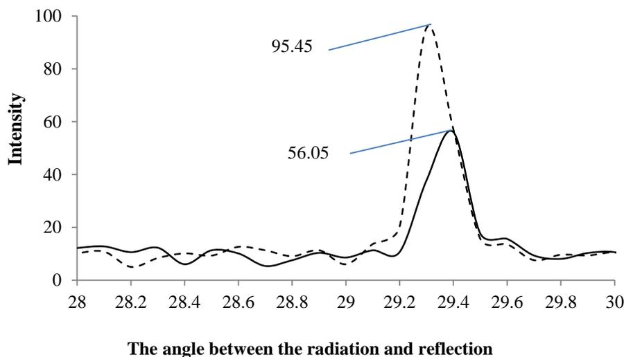
**Fig. 4.** X-ray diffraction diagram of colloid numbers 1 (fill line) and 2 (dashed line)
