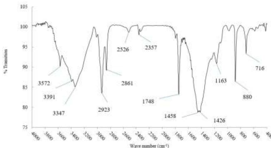
**Fig 3.** Colloidosome 2 infrared spectrum loaded with caffeine
