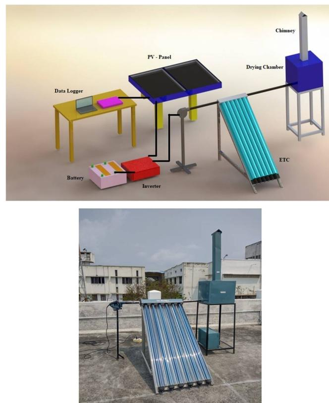
Fig. 1. Photovoltaic thermal hybrid solar dryer assisted with ETC, a). Schematic diagram and b). Photographic view
