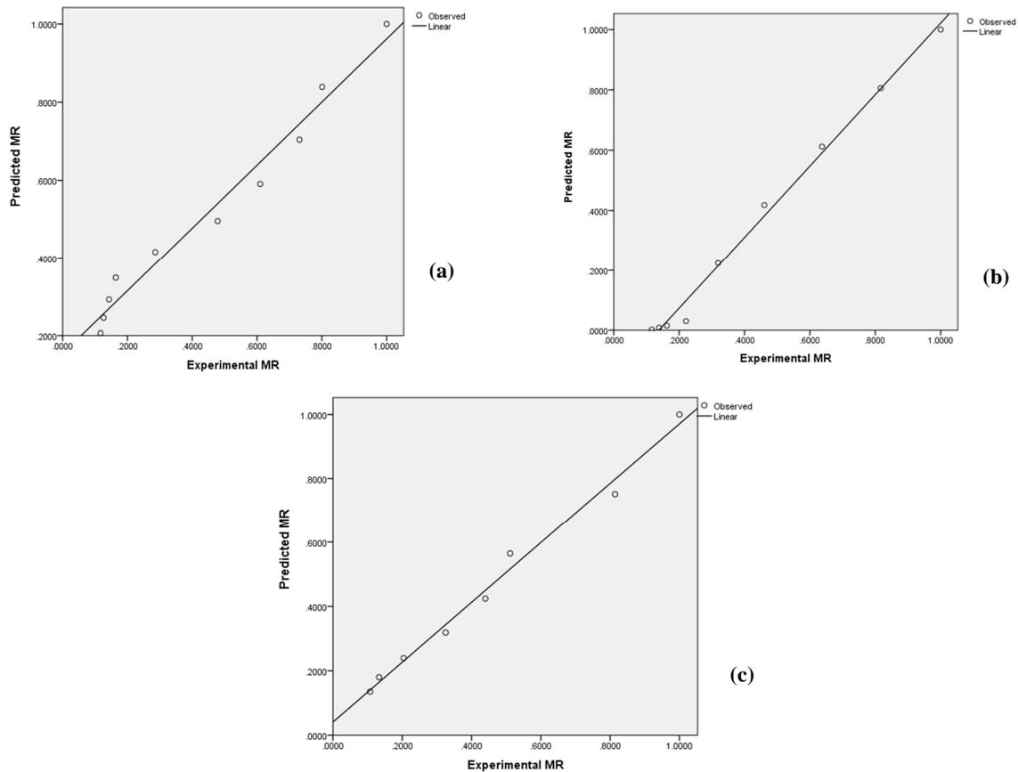
**Fig. 3.** Experimental vs predicted moisture ratio for drying of potato in the designed solar dryer; a) 50, b) 55, and c) 60 °c for Midilli *et al.* model
