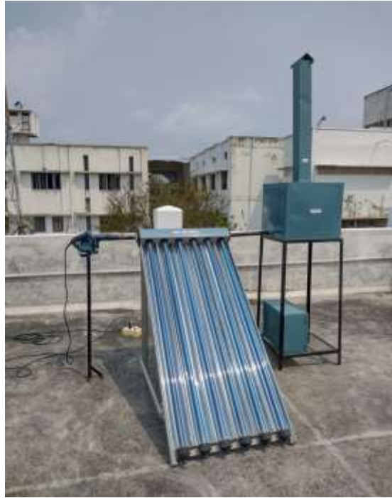
Figure 2.1(b). Photographic view of Photovoltaic Thermal Hybrid Solar Dryer assisted with ETC
