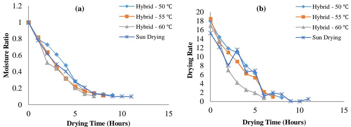
**Fig. 2.** a) Moisture ratio vs drying time for PV-T-hybrid solar dryer under various temperatures for untreated potato slices and b) Drying rate vs drying time for drying of untreated potato slices under various drying methods
