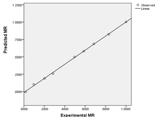
**Fig. 4.** Experimental vs predicted moisture ratio of drying of potato in traditional sun drying for Midilli *et al.* model
